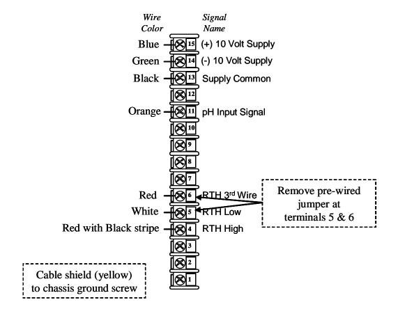
Figure 7-13 Terminal Designations for Durafet III Electrode with Cap Adapter
